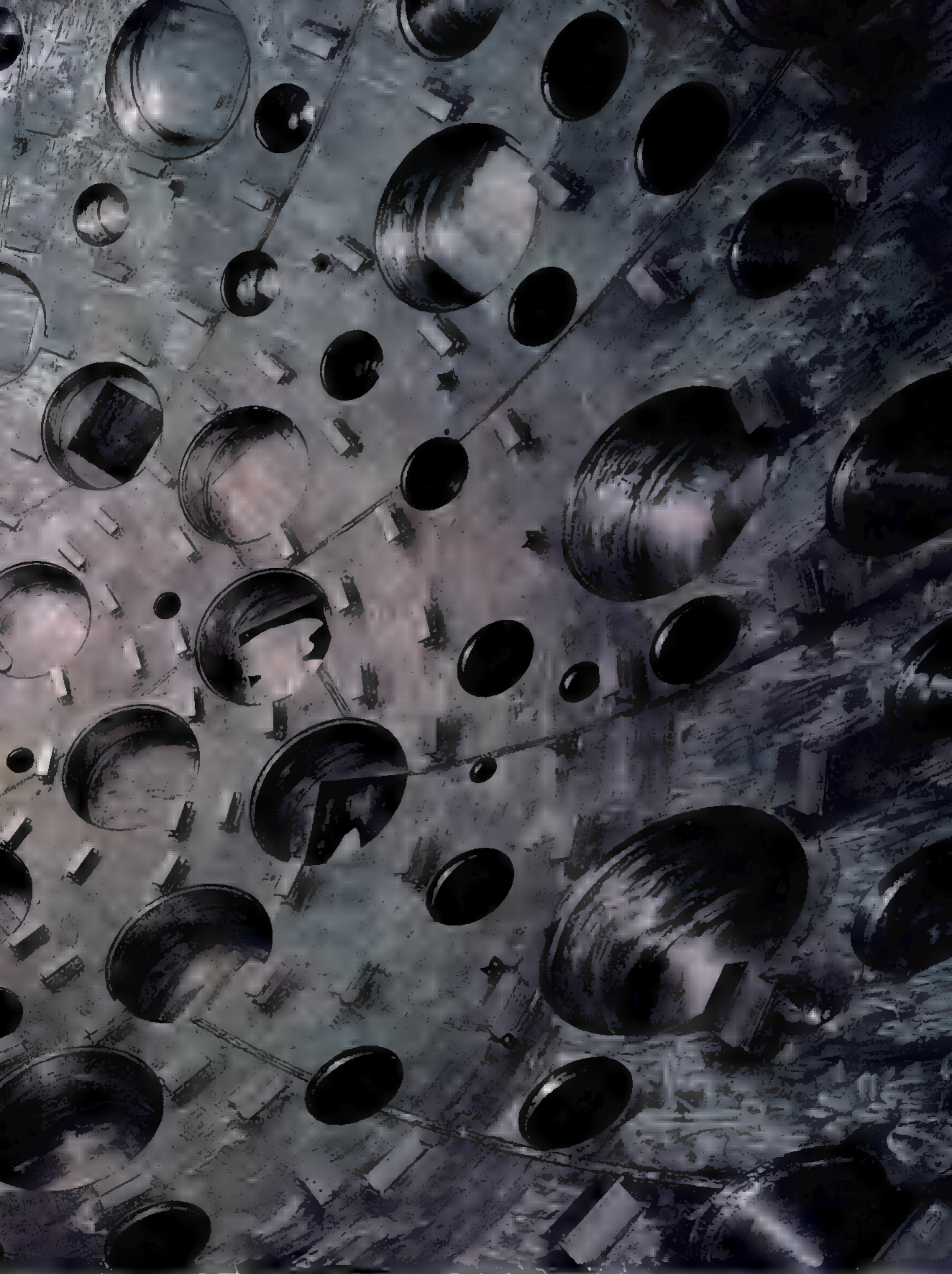
Creeping like a fly on a wall, Vaughn Draggoo inspects the huge target chamber at the National Ignition Facility in California, a future test site for light-induced nuclear fusion. Beams from 192 lasers will be aimed at a pellet of fusion fuel to produce a controlled thermonuclear blast.
